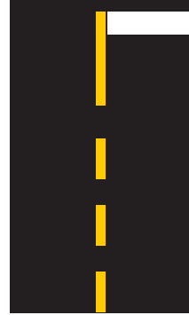
Stop line — stop before this line
