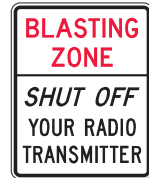
Blasting ahead — follow instructions on sign
