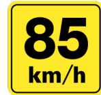
Indicates the recommended maximum speed through this curve under ideal driving conditions.
