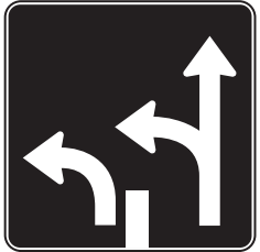
Side-mounted multiple lane designation
