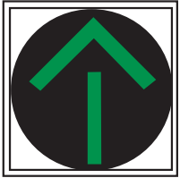
Steady through green arrow
