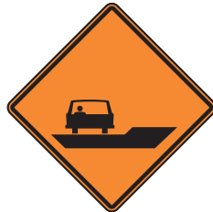
High shoulder ahead. Difference in elevation due to construction
