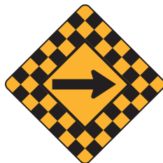
Sharp turn or bend in the roadway ahead
