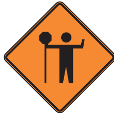
Traffic control person ahead
