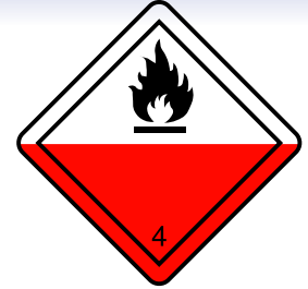
Class 4 Flammable Solids and Spontaneous Combustion
