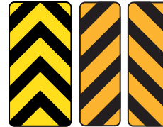
Hazard warnings Drive to the direction the slopes are pointing
